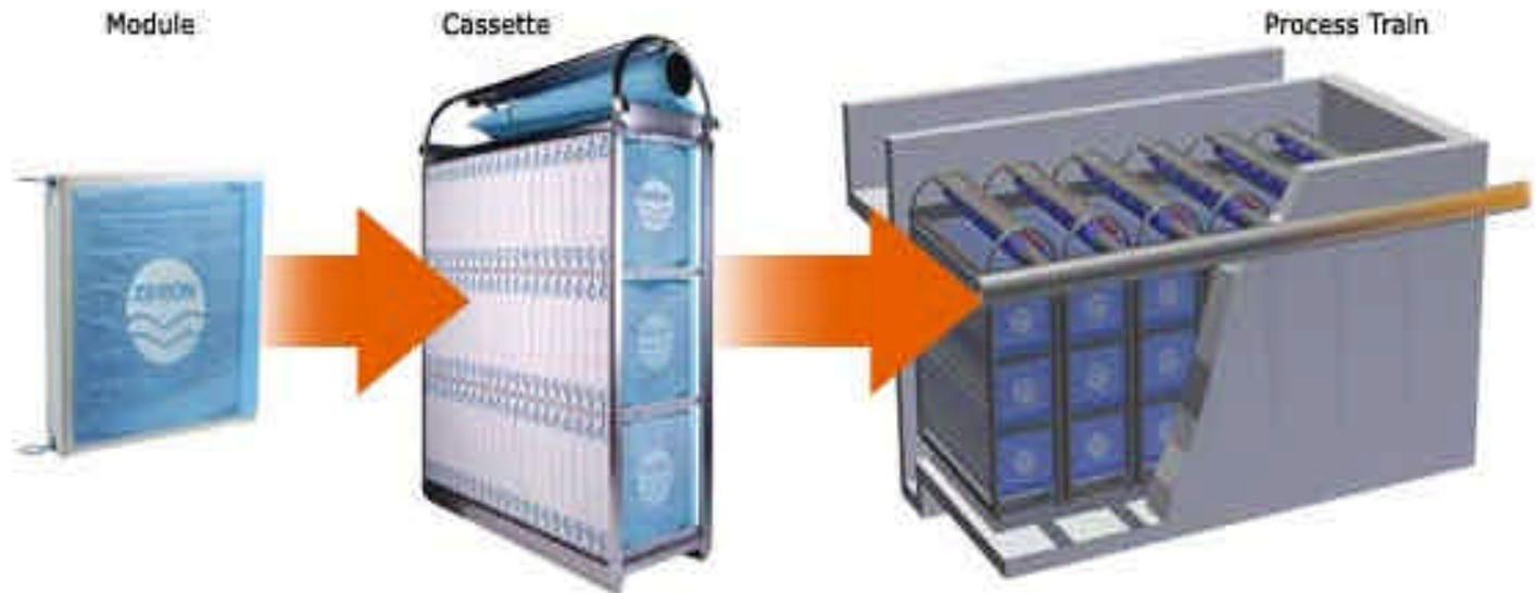
Filtration is achieved by drawing water to the inside of the membrane fiber under low vacuum pressure. The treated water (permeate) is conveyed to the main permeate collection pipes. The ZeeWeed 1000 Series membrane utilize "Outside-In" flow through a hollow-fiber membrane that has nominal and absolute pore sizes of 0.02 and 0.1 microns respectively. The small pore size excludes particulate matter including solids, bacteria, pathogens and certain viruses.
